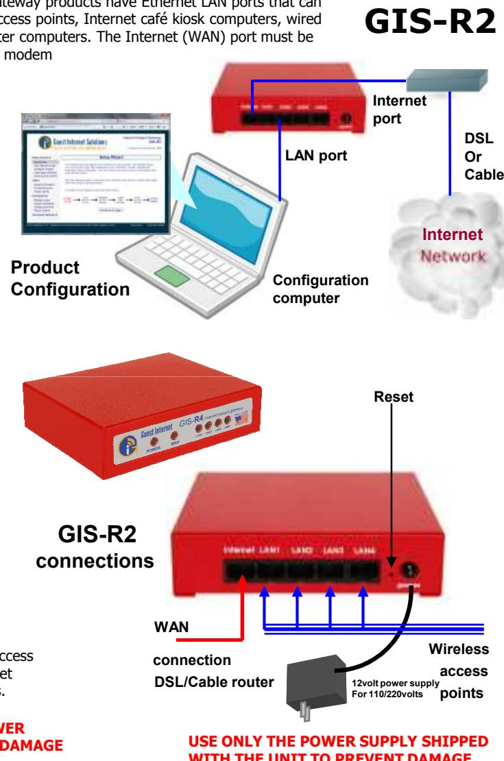
**Reset to Factory Defaults:** With the gateway powered up, use a paperclip to press the reset button through the hole shown. Hold the reset button down for 10 seconds then release. All parameters will be reset.
