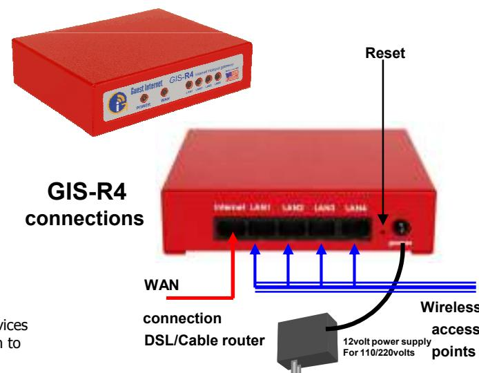
**Reset to Factory Defaults:** With the gateway powered up, use a paperclip to press the reset button through the hole shown. Hold the reset button down for 10 seconds then release. All parameters will be reset.
